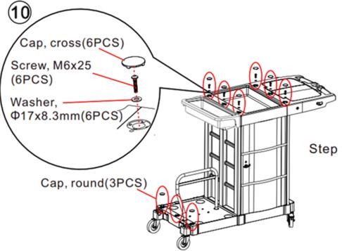
Step 10: Fasten the roof board and handrail board with screws. And put the cross cap in the roof board. Then put round cap in the bottom plate.
