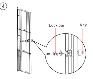
Step 4: Install the lock in the front door. Pay attention to set the lock bar perpendicular to the key.
