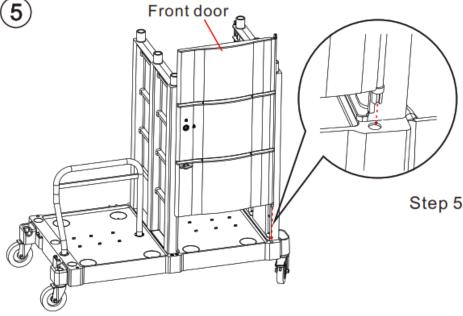
Step 5: Install the front door in the bottom plate.
