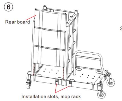
Step 6: Install the rear board in the bottom plate. Pay attention to set the rear board on the same side with the installation slots of mop rack.
