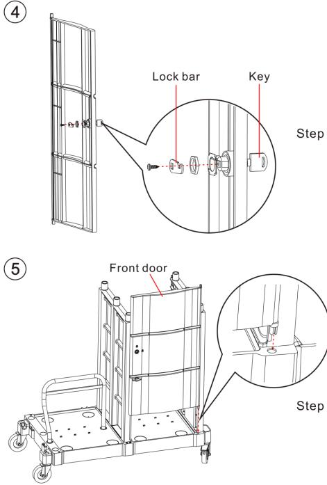
Step 4: Install the lock in the front door. Pay attention to set the lock bar perpendicular to the key.
