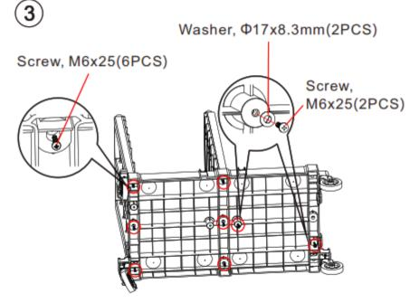
Step 3: Fasten side plates with screws. Then fasten the rack with washers and screws.
