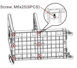
Step 3: Fasten the side plates with screws.
