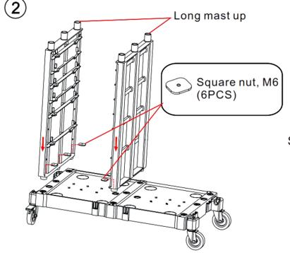
Step 2: Install the side plates on the side of castors with brake. Then insert the square nuts into the bottom of the side plates.
