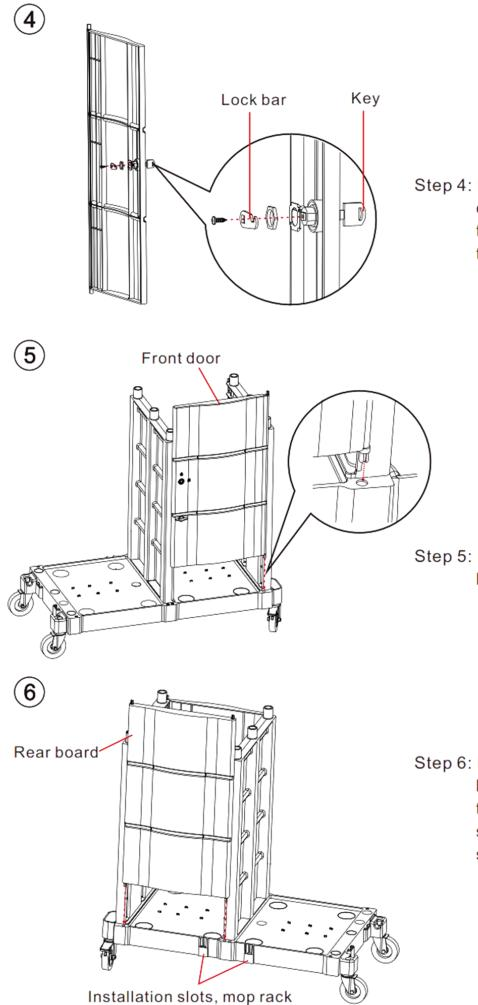
Step 4: Install the lock in the front door. Pay attention to set the lock bar perpendicular to the key.
